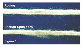
Loose ends of the cut fibres can be seen protruding from the surface of the yarns. The normal textile yarn forming process of fibre bale opening, carding, drawing, and spinning, by which these yarns are made, breaks some of the fibres into even shorter lengths, further aggravating the media migration problem.
